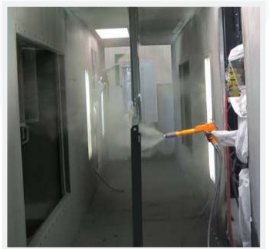
Parts being powder coated
