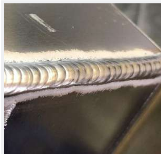
An example of a strong and visually pleasing aluminium TIG weld
