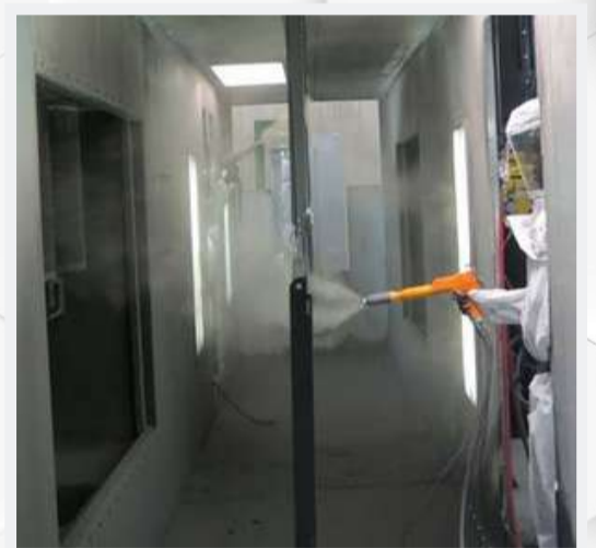
Parts being powder coated
