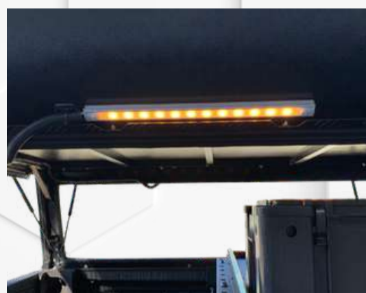
Amber light provides less visibility but doesn't attract insects
