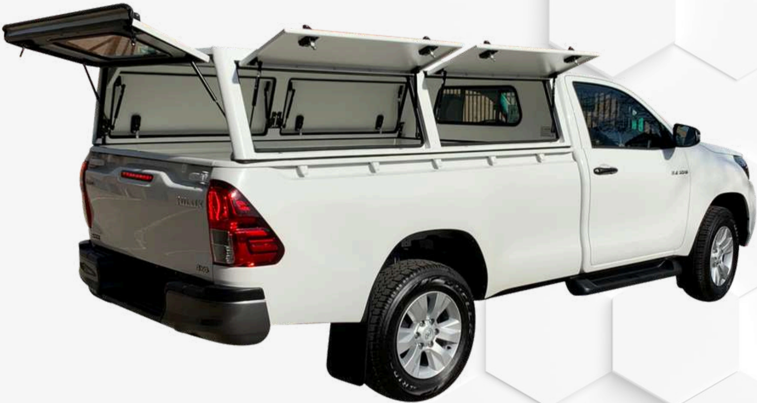
Five pop up doors for easy access to load bin
