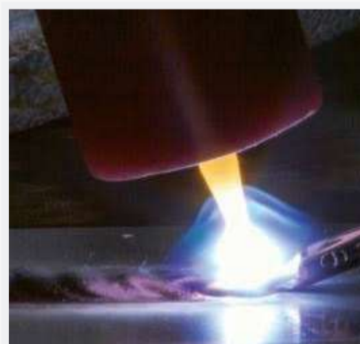
Water cooled TIG welders allow us to weld at a high current for added strength
